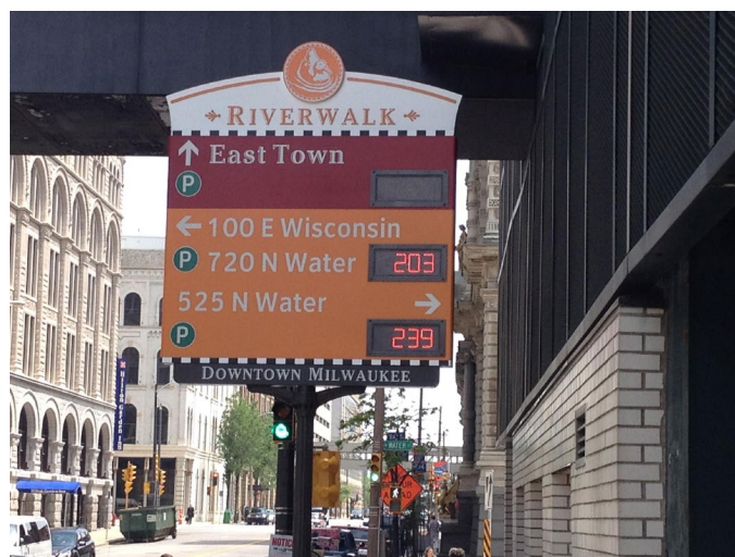
Example of an information board as part of a parking guidance system in downtown Milwaukee, WI. Photo: Scott Wise
